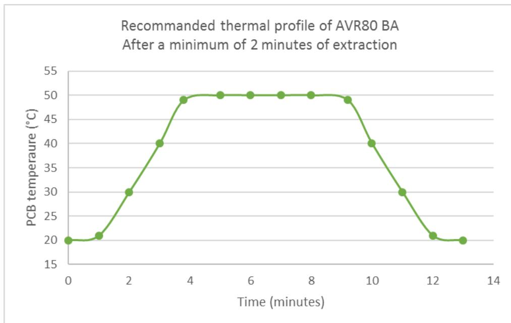
This thermal profile can be adapted:  $\pm 10^{\circ}\text{C}$ , depending some more parameters, such as: thickness deposit, design of the PCB...
